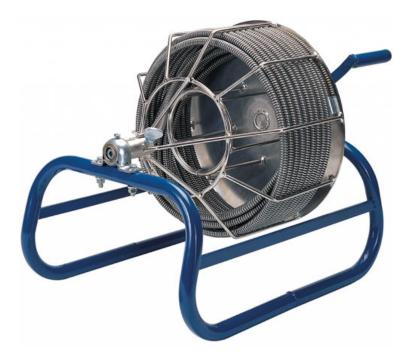
The Model K is a high-quality manual unit that quickly clears clogged pipelines and makes pipeline maintenance quick and easy. The Model K is a professional quality, manual unit for cleaning 1 1/4? – 3? diameter lines up to 100ft. The heavy-duty frame is reinforced on both sides for added durability. The cable cage is powder coated to resist rust.
