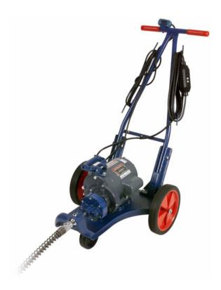
The Model C Sectional Drain Cleaner is the best unit available for tougher blockages such as tree roots and for longer runs in main sewer lines. The Model C runs up to 200ft. of 1 1/4? dual cables, with self-feeding action, that are available in 8ft. sections for cleaning 3?-10? diameter lines. The standard 1/2HP motor spins the cable at 500 RPM for maximum cleaning power.
