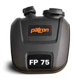
This water tank is designed to be used with Patron FP75 and FP100 plate compactors. When compacting hot asphalt, a constant supply of cool water is needed on the surface to avoid hot asphalt sticking to the cold plate of the compactor. Water tanks are also ideal for very dusty applications.
