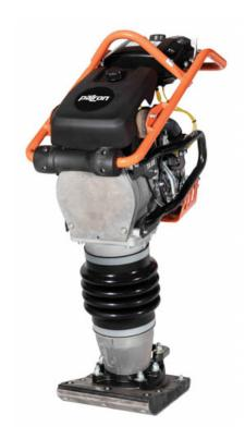
The TA65 is our largest rammer with an 11" wide base plate. This machine features the highly adept and purpose-built Honda GXR120 rammer engine that is designed to persist through the most difficult compaction conditions. Patron rammers are built with high quality components and are designed with easy access to service points, so most maintenance can be done on site. The slim handle makes this unit perfect for jobs in tight quarters.
