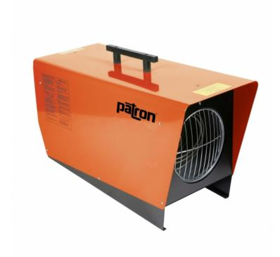
The Patron 18E-1 is a compact, yet powerful source of clean, dry heat. This unit produces 65,000 BTU/Hr and disperses heat across a large area with a 590 CFM fan. Useful in any application from construction sites to tented events, the 18E-1 is extremely safe and reliable. Be advised this is the single phase version, which requires 81 amps to operate.
