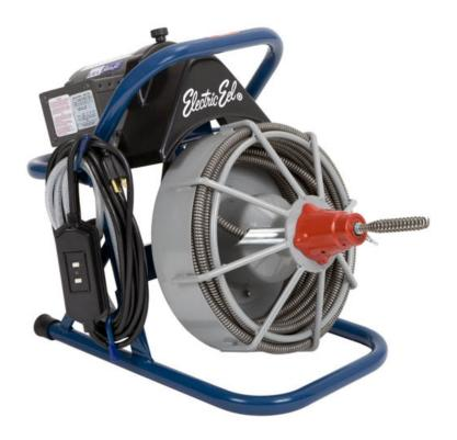
Designed specifically for the rental industry, the Model E has several unique features such as a steel inner-drum, epoxy coated cage, cord wraps, and a rear bar for motor protection. Unit holds up to 75 Ft. of 3/8? or 1/2? diameter "galvanized aircraft wire" inner core. Cleans 1 1/4? – 3? diameter lines. An optional 2 wheel dolly is available for easy transport.
