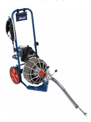
The Z5 cleans 1-1/4" - 3" diameter lines up to 75 ft. and fills the gap for those jobs that require a longer run in smaller drain lines. The auto-feed function allows the operator to advance and retrieve the cable with the push of a lever. The cable runs through a guide spring which keeps hands off the rotating cable for added safety.
