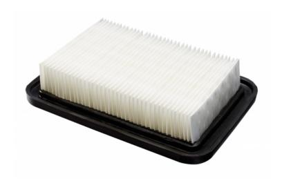
The Milwaukee 49-90-1953 main filter replacement is compatible with the Milwaukee 8-Gallon Dust Extractor (8960-20). It's PTFE membrane provides 99.9% efficiency for tough dust producing applications and is a washable filter.
