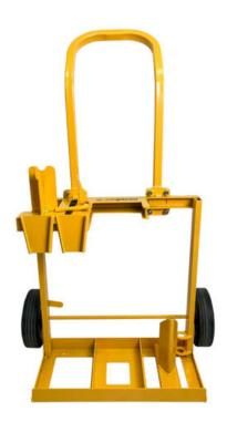
A nice way to keep the Panellift®, well, nice! Load the disassembled lift onto the cart and then it can be easily moved around a jobsite or loaded onto a company vehicle. The 117 storage cart works with the model 138-2, 125, and 439. All-steel material, made in the USA.
