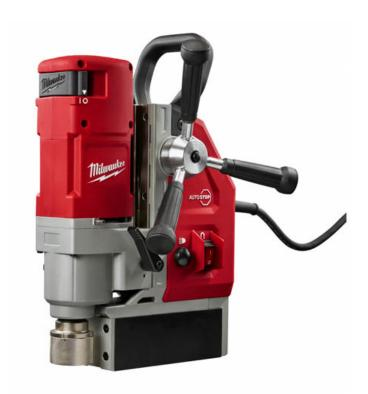
The Milwaukee 1-5/8" Electromagnetic Drill delivers the faster set-up, cutting and drilling. It's 13 amp motor delivers the fastest drilling w/ annular cutters or twist drill bits. Equipped with a 2-speed gear box the tool can be adjusted tool-free between annular cutters at 475RPM and twist drill bits at 730 RPM.
