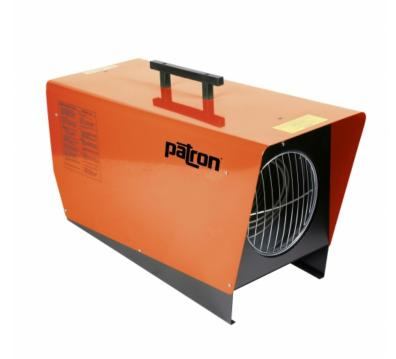
The Patron 18E-3 is a compact, yet powerful source of clean, dry heat. This unit produces 65,000 BTU/Hr and disperses heat across a large area with a 590 CFM fan. Useful in any application from construction sites to tented events, the 18E-3 is extremely safe and reliable. Be advised this is the 3-phase version, which requires 240V 3-phase power.
